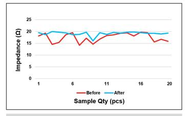
Very consistent OCV/CCV. No obvious differences on impedance between cells post 85C/85%RH test.
