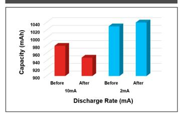
Almost no difference in low rate 2mA capacity. High-rate 10mA capacity retention is good (can reach 92%).
