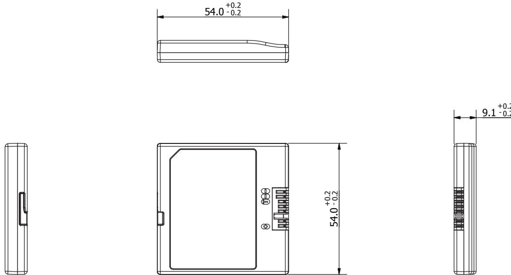
(1) Dimensions are in millimetres. (2) Consult Accutronics for device cavity design advice
